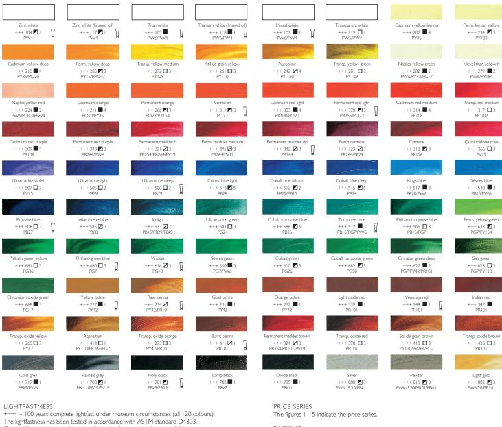
The lightfastness has been tested in accordance with ASTM standard D4303. Colours illustrated approximate to the real colours as nearly as possible.
